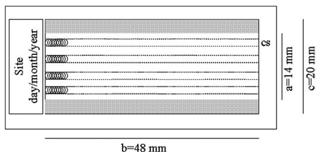
**Fig. 1** Scheme of a daily slide:  $a \times b$  = standard sample area after the standard UNI 11108:2004 (or central area of the tape);  $c \times b$  = adhesive tape (or whole sampling surface); routine scheme adopted by the aerobiological centre of San Michele a/A for the counting: 4 continuous sweeps (cs) at 400 $\times$ , diameter of microscope field = 0.5 mm.
